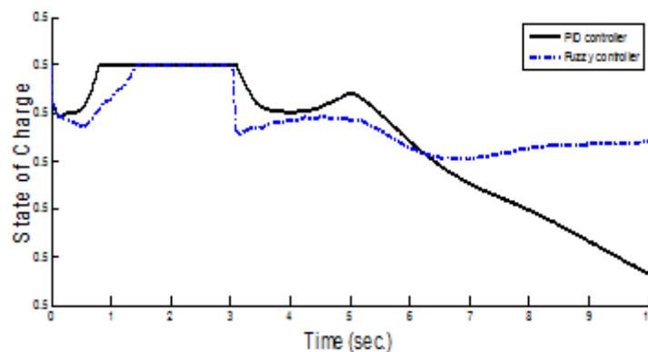
Figure 7: The rate of charge and discharge of battery
