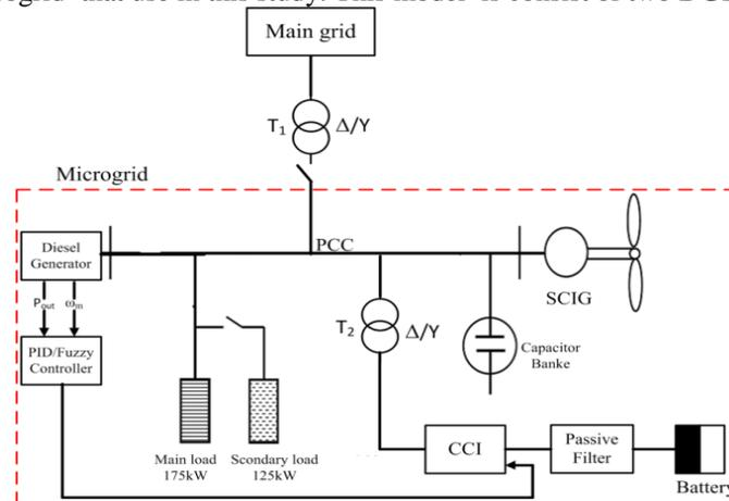
Figure 1: Microgrid Model
