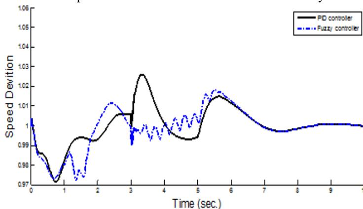
Figure 4: Changes speed of synchronous machine
