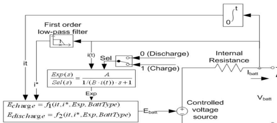
Figure3: Battery model lead acid type in Matlab/Simulink
