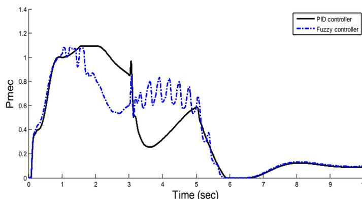
Figure 5: Mechanical power of synchronous machine
