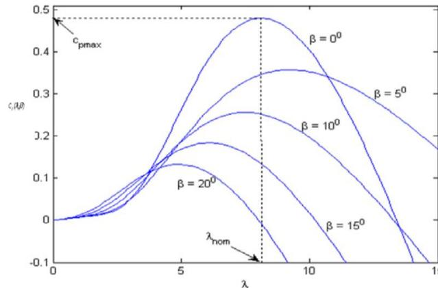
Figure 2: Performance coefficient  $C_p$  as a function of the tip speed ratio  $\lambda$  with pitch angle  $\beta$  as a parameter.
