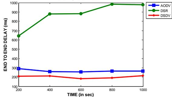
Figure 10. Average End-to-End Delay of Routing Protocols
