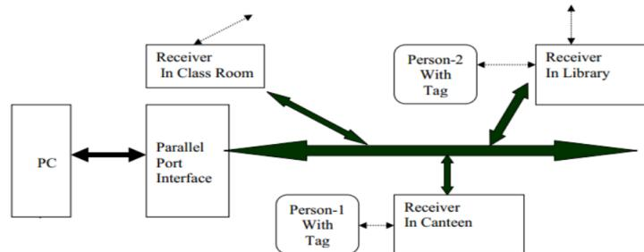
Fig 1: RFID Based Object and Location Identification Tool System Architecture
