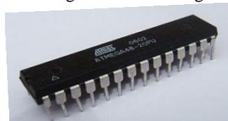
Fig 2: Atmega48 Micro controller
