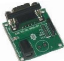
Fig 4: RFID Reader Module
