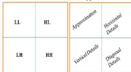
Fig.3 Final stage of step 1 wavelet decomposition
