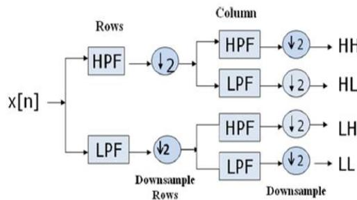
Fig.4 Block diagram of 1 step 2-D DWT
