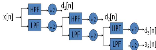
Fig.1 Wavelet decomposition tree (Three-level)
