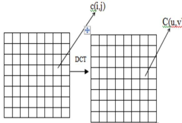
Fig-7 Discrete Cosine Transform of an Image
