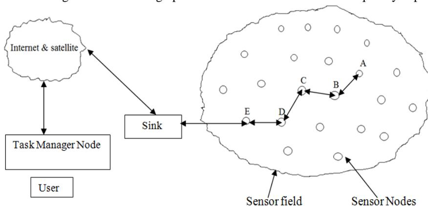
Figure 1: Communication Architecture of Wireless Sensor Networks
