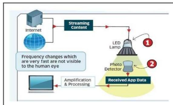
Fig 4: Block Diagram of Li-Fi system.
