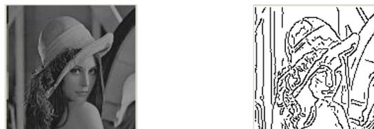
Fig2 (a): original image Fig2 (b): Image with edge Detected
