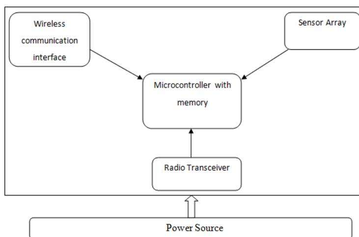
Fig. 2: Block Diagram of components of a Sensor Node
