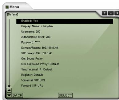
Fig.X-litesoft phone at the client's end, along with its configuration
