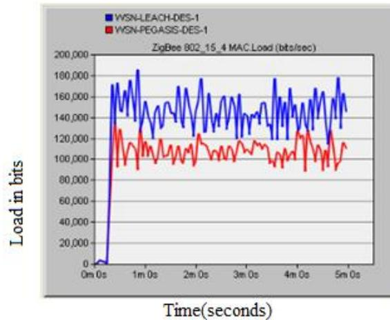
Fig 5.3: Data traffic rcvd(bit/sec)
