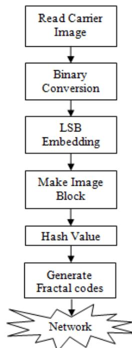
Fig. 3 Block Diagram of Proposed work at sender end.
