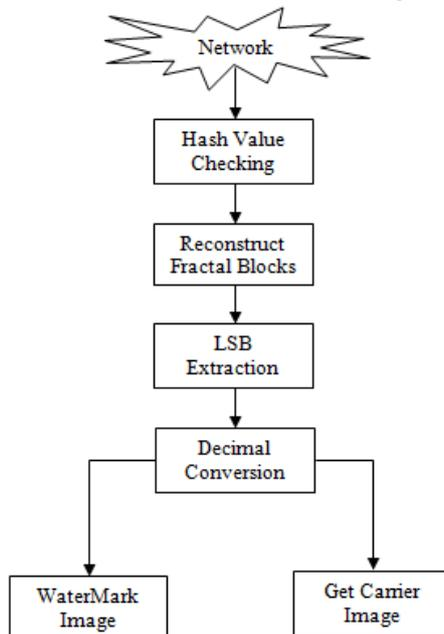
Fig. 4 Block Diagram of Proposed work at sender end.
