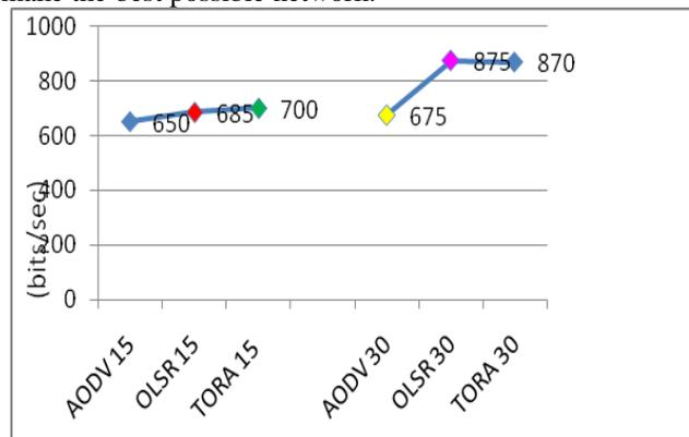
Figure .8 Measurements of Network Load with 15 and 30 nodes
