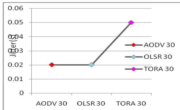
Figure 10 Measurements of Jitter(s) with 30 nodes
