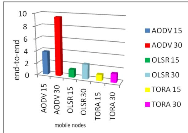
Figure.7: Delay comparison in routing protocols with 15 and 30 nodes
