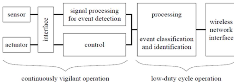
Figure 2. Architecture of Wireless sensor Network
