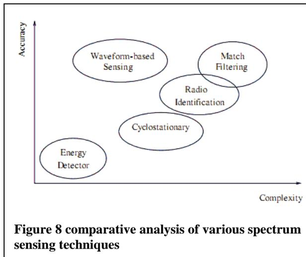
Figure 8 comparative analysis of various spectrum sensing techniques
