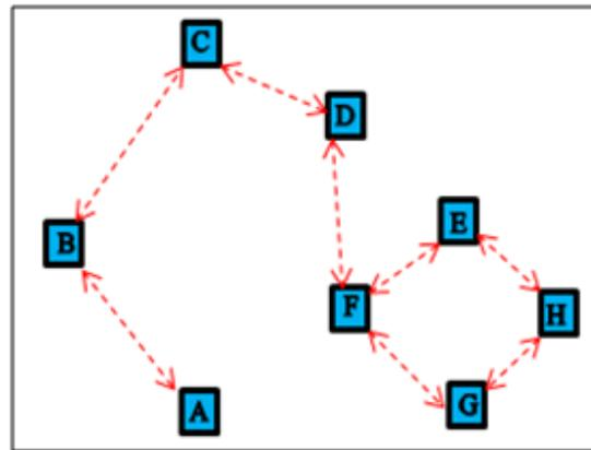
Figure 4: DSDV Protocol Structure
