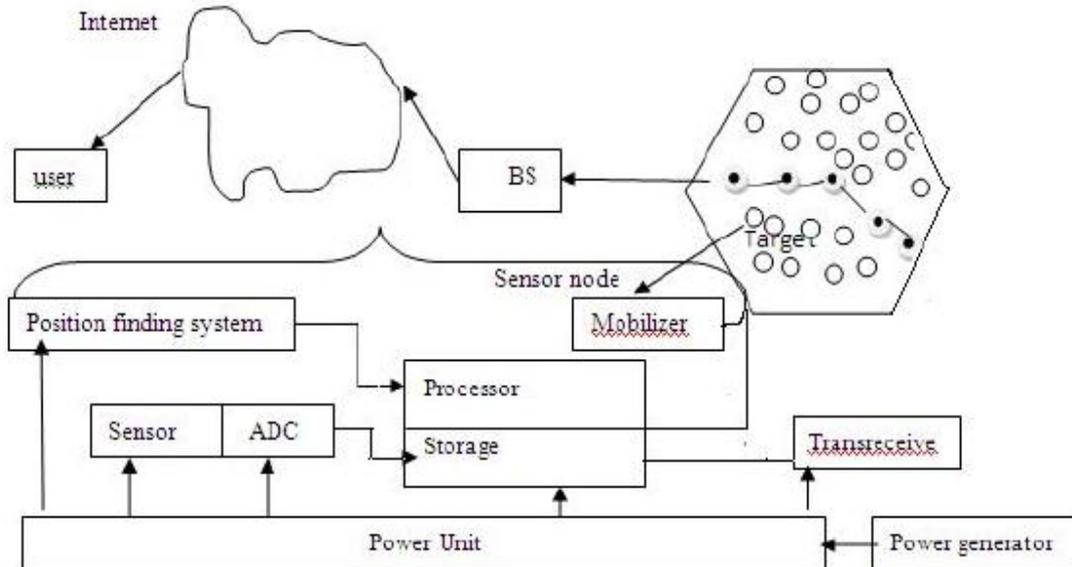
Figure 2 .Sensor nodes scattered in a sensor field and components of a sensor Node
