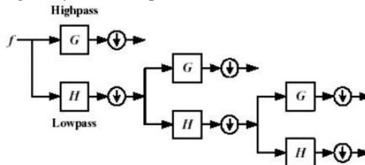
This decomposition halves the time resolution since only half the number of sample now characterizes the whole signal. Frequency resolution has doubled because each output has half the frequency band of the input. This process is called as sub band coding.
