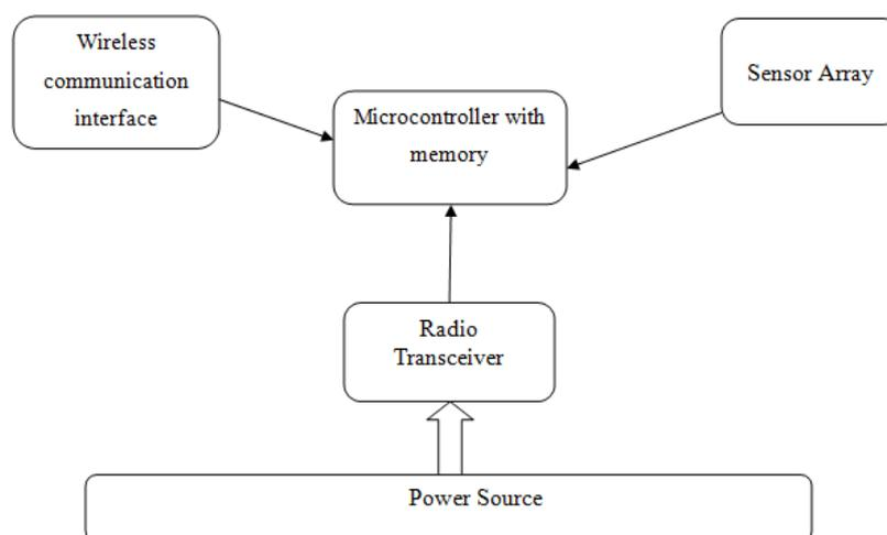
Fig. 1.2 Block diagram of a typical Wireless Sensor Node
