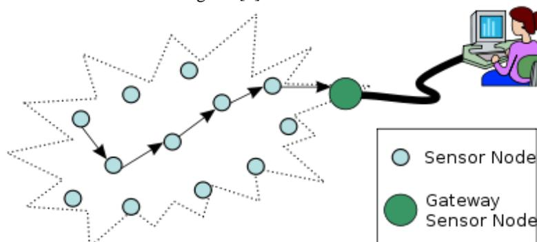
Fig. 1.1: Typical multi-hop wireless sensor network architecture
