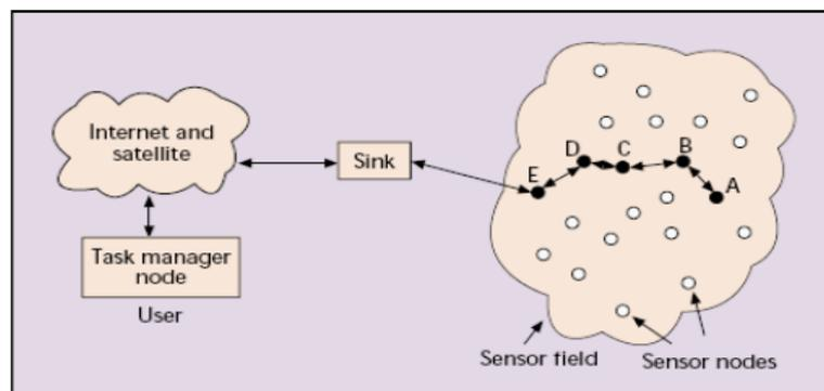
Fig 1 View of a wireless sensor network [19]
