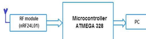
Fig. 3(c) Block Diagram of Receiver-end
