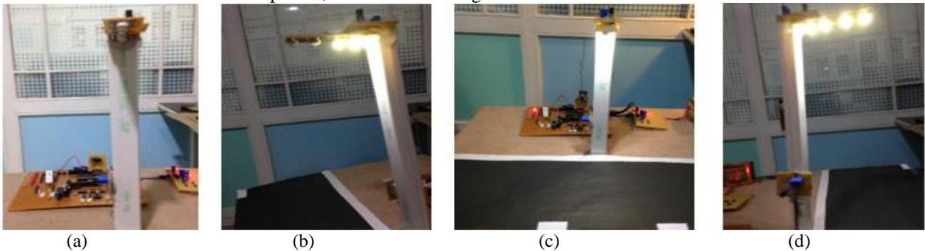
Fig. 5 (a) Lamp is OFF during day light, (b) Half of the LEDs of Lamp turns ON detecting night, (c) Variation in intensity of Lamp according to LDR1 and LDR2, (d) All LEDs of Lamp turns ON detecting vehicle.
