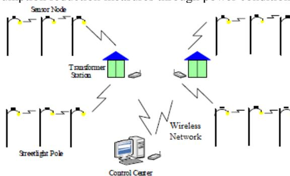
Fig.1 Structure of streetlight power cable monitoring system based on wireless sensor networks
