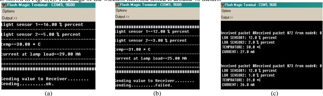
Fig. 6 (a) Sending Ok for transmitting information at transmitter terminal of the system, (b) Sending Failed for transmitting information at transmitter terminal of the system, (c) Receiver terminal for monitoring the system.
