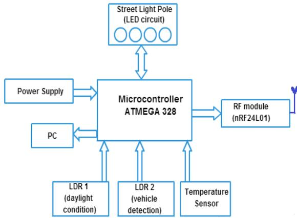
Fig. 3(a) Block Diagram of Transmitter-end on the Pole
