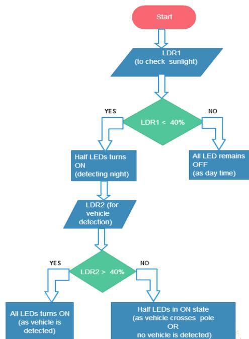
Fig. 4 Flowchart of the Proposed Intelligent Street Light System
