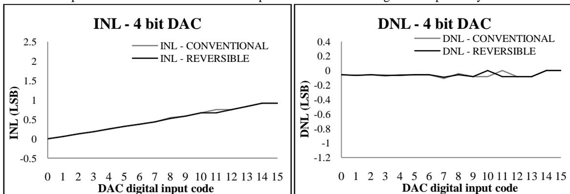
Fig. 6 INL and DNL analysis of 4-bit R2R DAC considering conventional and reversible logic based implementations
