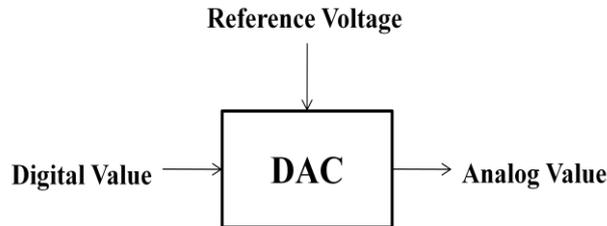
Fig. 1 Functional block diagram of Digital to Analog Converter (DAC).
