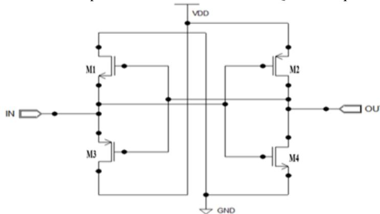
Fig. 4 Reversible CMOS Inverter using QFG Technique
