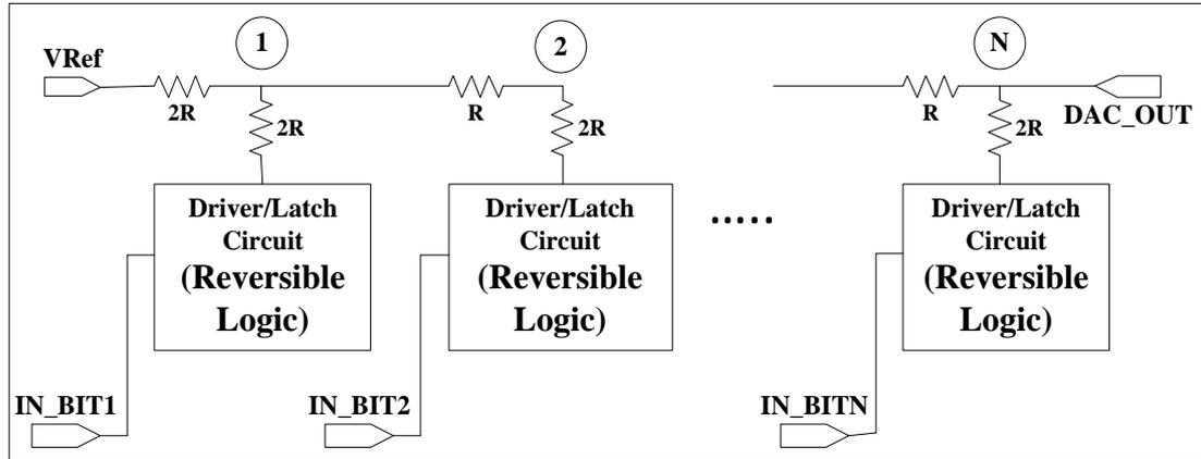
Fig. 3 N-bit Reversible R2R DAC
