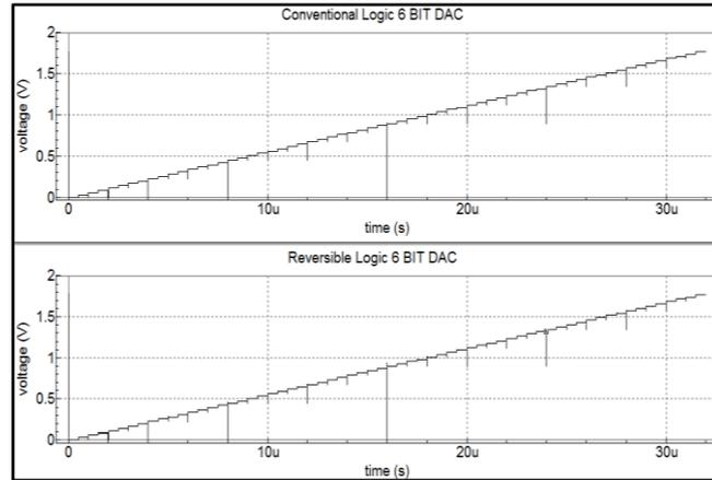
Fig. 7 Transient response of 6-bit R2R DAC considering conventional logic and reversible logic
