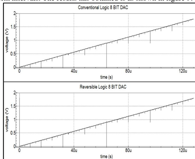
Fig. 9 Transient response of 8-bit R2R DAC considering conventional logic and reversible logic
