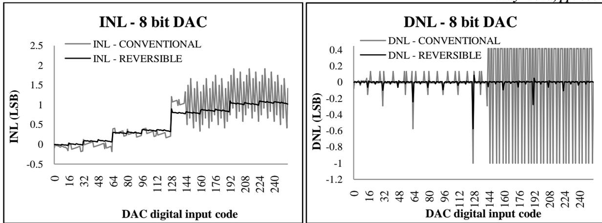
Fig. 10 INL and DNL analysis of 8-bit R2R DAC considering conventional and reversible logic based implementations
