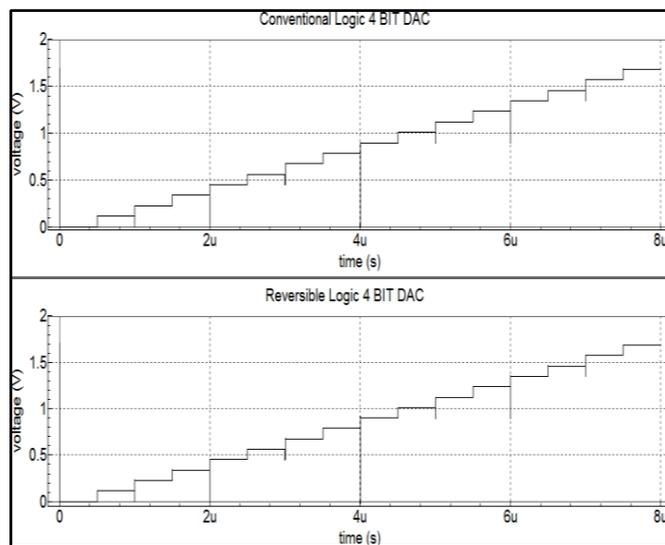
Fig. 5 Transient response of 4-bit R2R DAC considering conventional logic and reversible logic.
