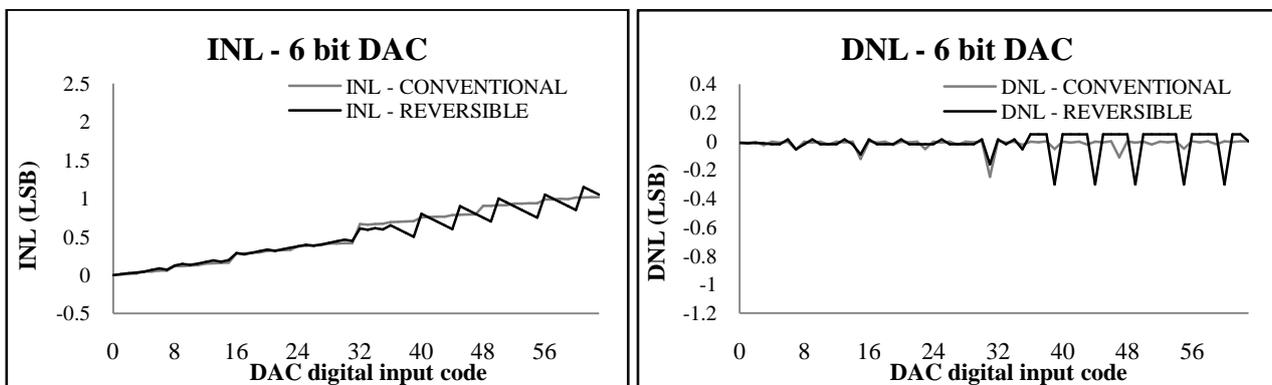
Fig. 8 INL and DNL analysis of 6-bit R2R DAC considering conventional and reversible logic based implementations
