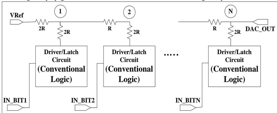
Fig. 2 N-bit Conventional R2R DAC
