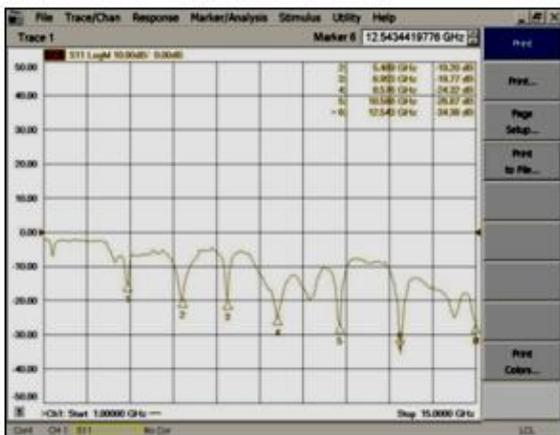
Fig. 4. Variation of return loss versus frequency of CCPARS
