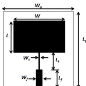
Fig. 1. Top view geometry of conventional RPA
