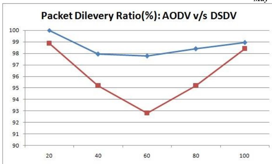
Fig. 1 Comparative analysis of PDR for AODV v/s DSDV against speed for MANET
