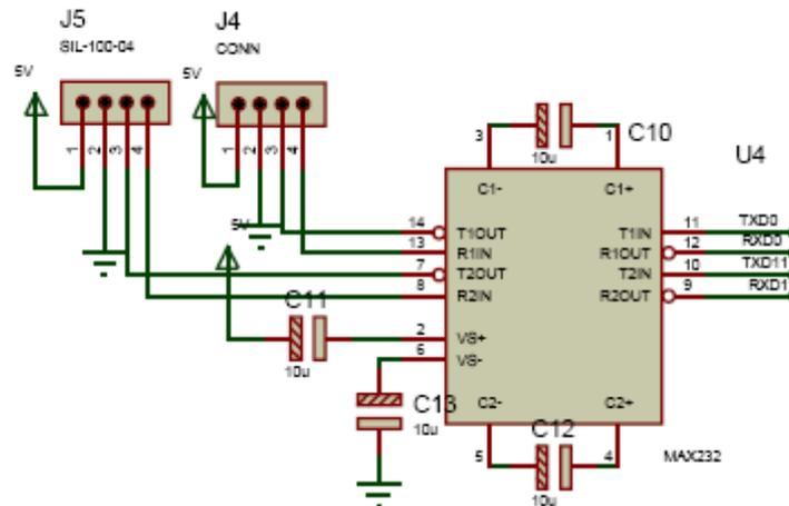
RS 232 IC is a driver IC to convert the  $\mu$ C TTL logic (0-5) to the RS 232 logic (+-9v). Many device today work on RS 232 logic such as PC, GSM modem, GPS etc. so in order to communicate with such devices we have to bring the logic levels to the 232 logic (+-9v).
