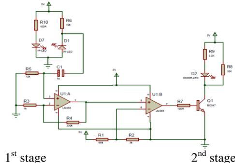
On the receiver side we have connected the IR receiver in reverse bias. So as soon as the light falls in the IR receiver, the anode voltage increases and when the anode voltage is more than the cathode voltage then the LED is in forward bias mode and start conducting.
