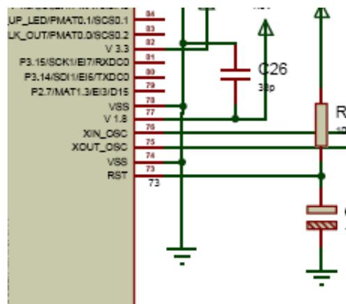
As shown in the above circuit we are connecting an RC circuit to the RESET (pin 57) of  $\mu$ C. The ARM  $\mu$ C has an active low reset, therefore we connect an RC circuit. As shown the capacitor is initially at 0v. It charges via the supply through a 10 k ohm resistance in series, therefore the reset time of our circuit is:
