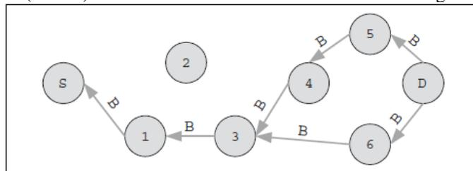
Fig. 3 Route Discovery Phase: The backward ant (B) is send by the destination node toward the source node [3]
