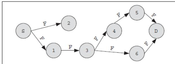
Fig. 2 Route Discovery Phase: A sender (S) sends forward ant (F) toward the destination node (D). [3]
