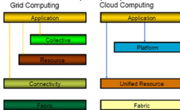
Figure 2: Grid computing and Cloud computing Architecture [2]
