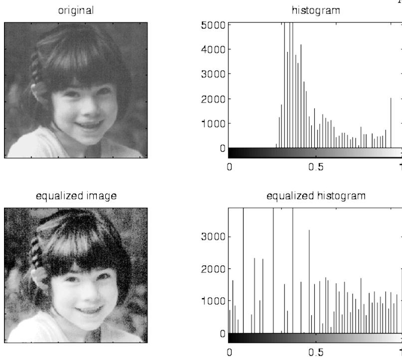
Fig. No. 2 Image Enhancement by histogram equalization
