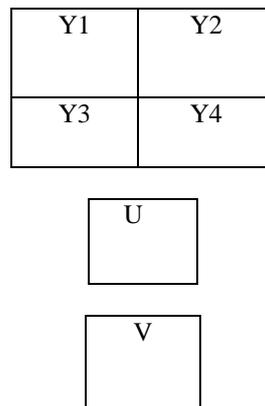
1.(a) With each macro-block (MB), information related to four luminance blocks ( $Y1, Y2, Y3, Y4$ ) and two chrominance blocks ( $U, V$ ) is coded. Each block contains  $8 \times 8$  pixel
