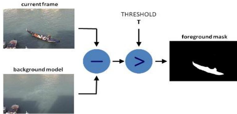
Fig. 3 Example of Background subtraction method
