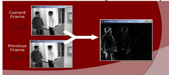
Fig. 2 Example of frame difference method
