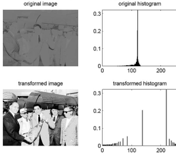
Fig 4: histogram equalization applied to low contrast image
