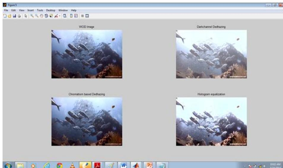
Fig 6: comparison between WCID and other underwater image enhancement techniques a) WCID image b) Dark channel dehazing image c) chromatism based dehazing image d) histogram equalization image
