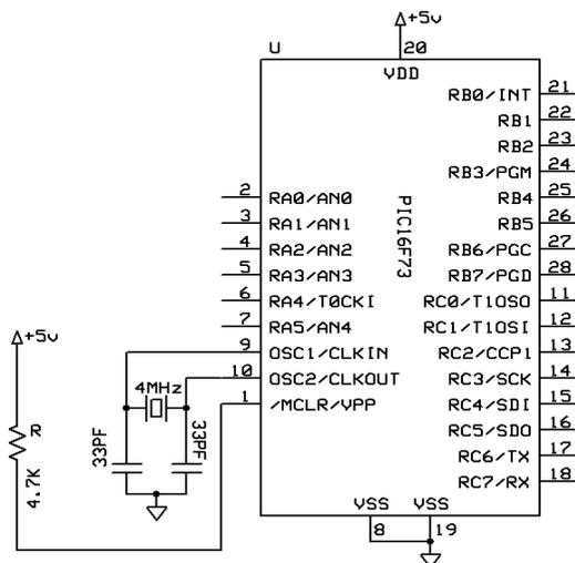
Fig 3.3: Microcontroller unit
