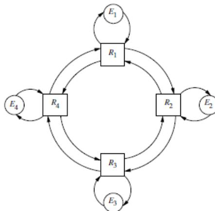
Fig. 3. The physical topology of a typical WDM network with four end nodes E1... E4 and four routers R1... R4
