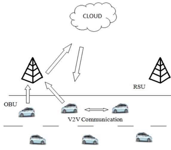
Fig 2: VANET using Cloud Architecture
