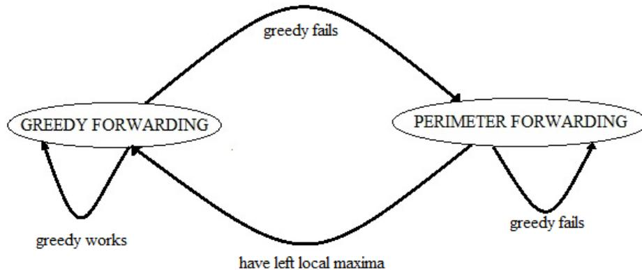
Fig. 1 Greedy Perimeter Stateless Routing (GPSR) Protocol
