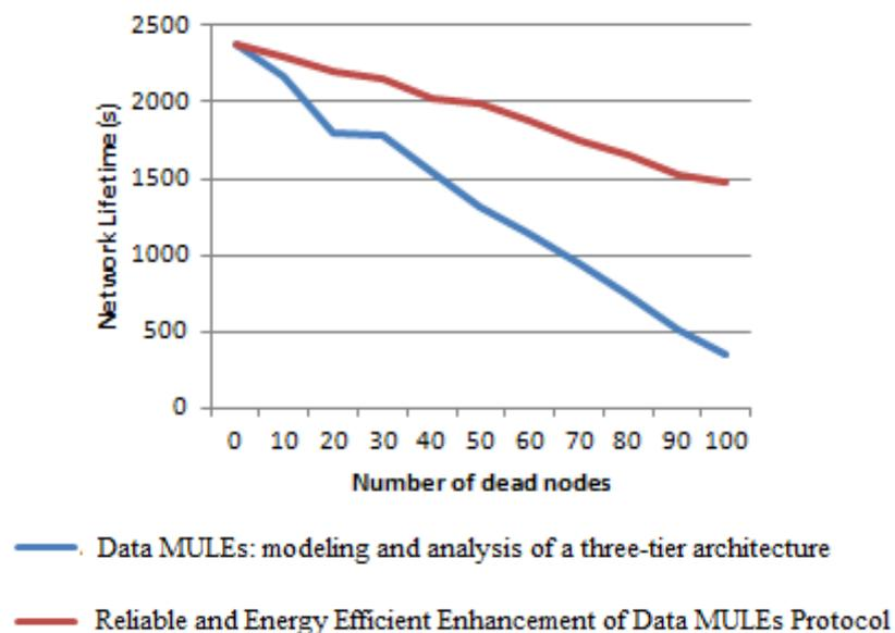
Fig. 8 Comparing Network Performance between Reliable and Energy Efficient Enhancement of Data MULEs Protocol and Data MULEs: modeling and analysis of a three-tier architecture in WSN to show the Network Lifetime. From Fig. 8, it can be observed that on implementing our algorithm the network lifetime increases.
