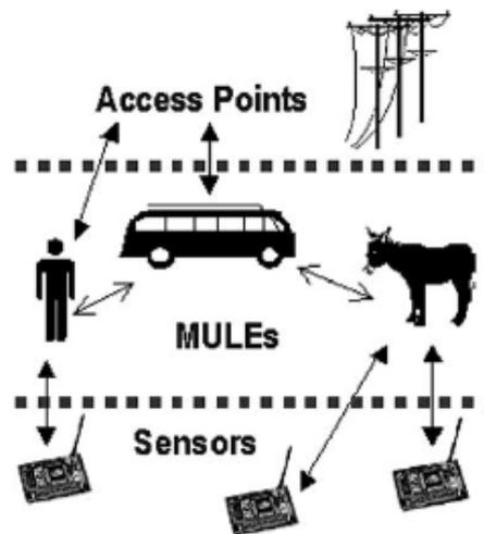
Fig. 4 The MULEs three tier architecture
