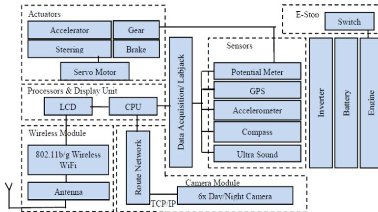
Fig.1 LANDARC's SPORV instrumentation and control sub-modules.
