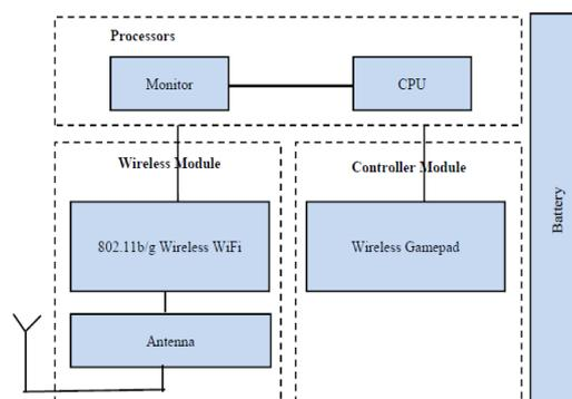
Fig. 2 Sub-modules of LANDARC's remote operator module
