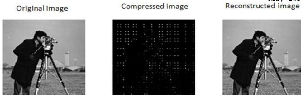
Fig.2 DCT compression of cameraman image
