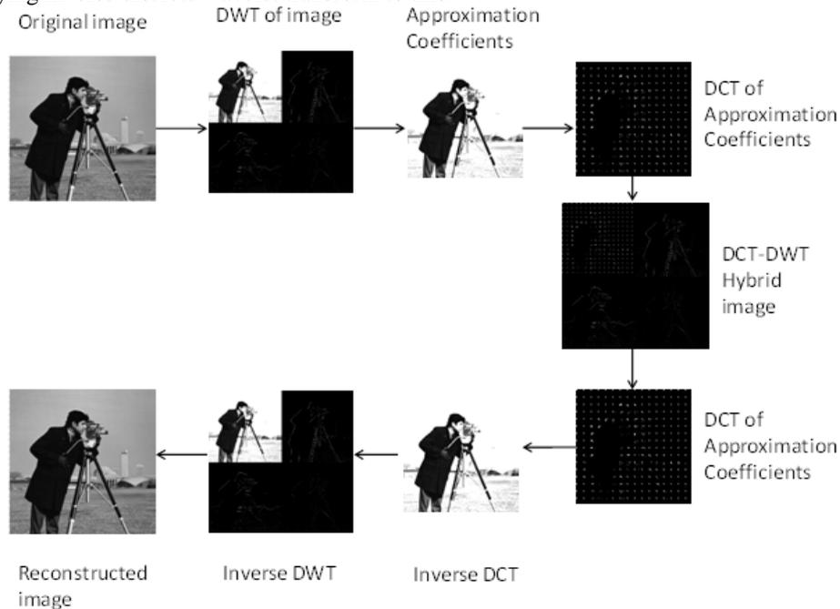
Fig.1 DCT-DWT Hybrid image compression technique block diagram.
