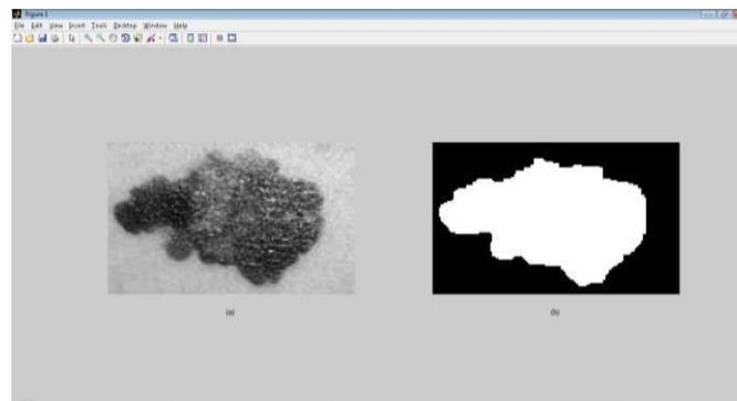
Figure 2:a) grayscale version of RGB, b) segmented image after applying Otsu method
