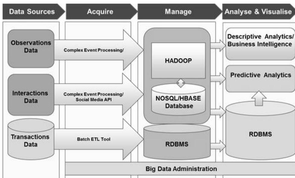
Fig.8: A high level typical Big Data solution architecture
