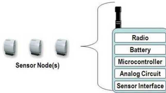
Figure:- 2 component of sensor node
