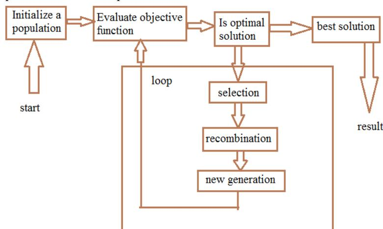
Fig. 4 structure of evolutionary algorithm
