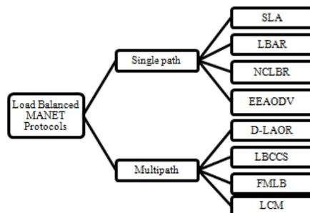
Fig.. 1 Classification of Load Balanced MANET Routing Protocols
