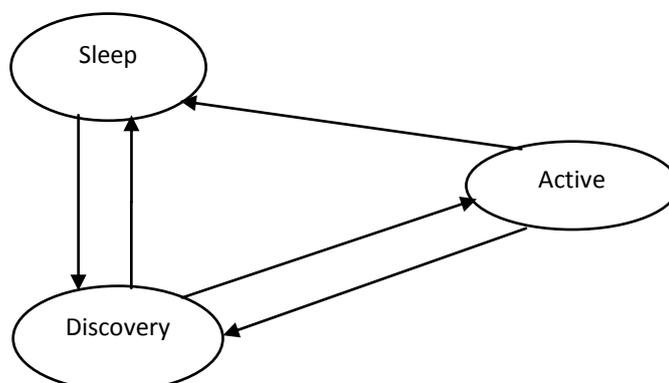
Figure 2.1.1: State Transition Diagram for GAF
