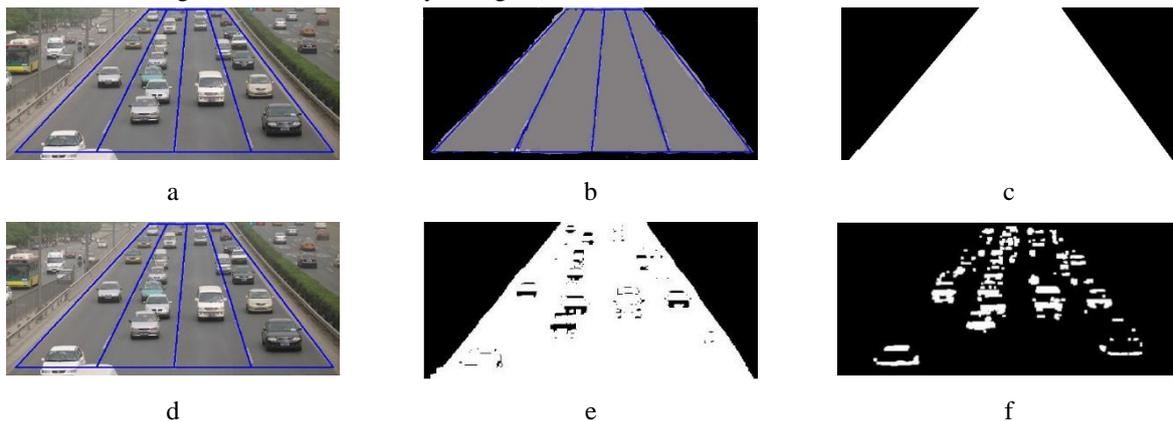
Fig. 2: Example of analysed image for a ROI. a) & d) are the original image, b) original image for the ROI background, c) binary mask for the ROI, f) classified vehicles.
