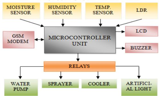
Fig. 4 Block diagram of proposed system hardware
