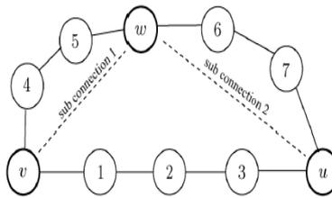
Fig3: Breaking a TCP Connection into two sub-connections reducing the maximum RTT.
