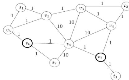
Fig1: Overlay routing example: Deploying relay server on v6 and v7 enables overlay routing.
