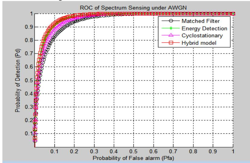
Fig.5 The ROC curves of hybrid model, matched filter, energy detector and cyclostationary detection.
