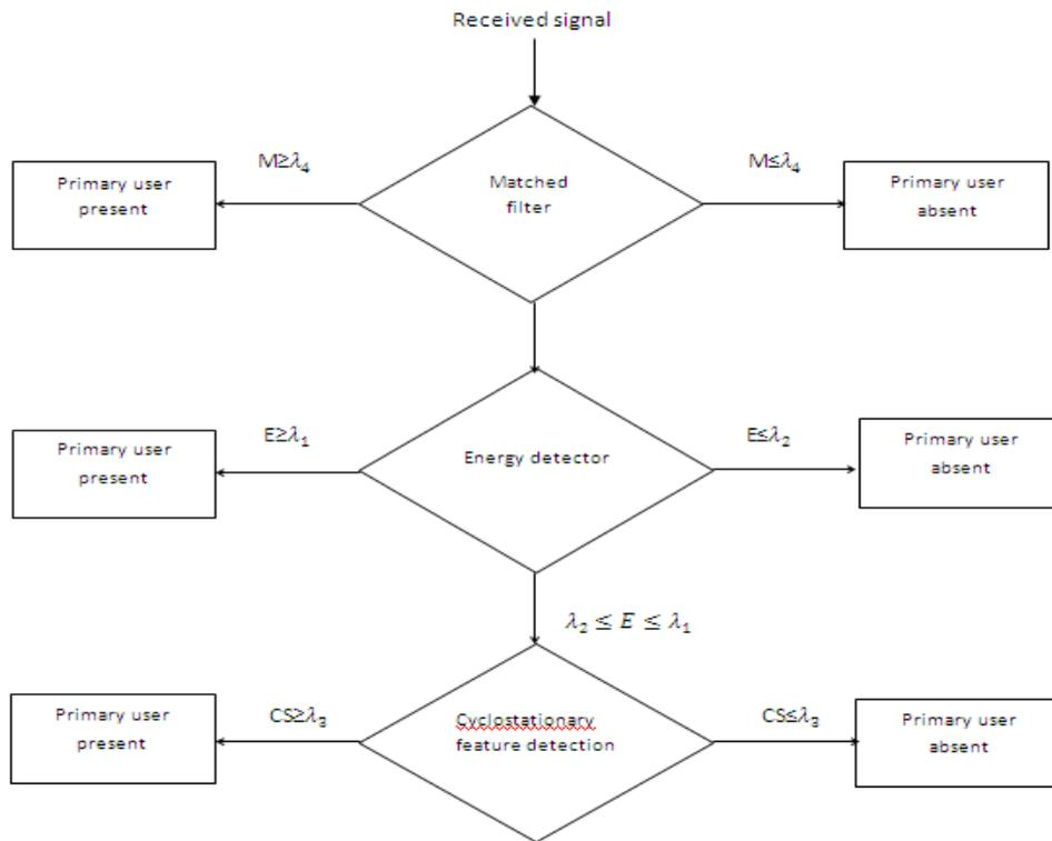
Fig.1 Hybrid model for spectrum sensing.
