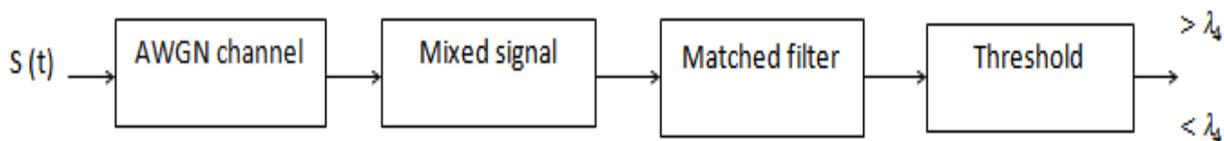
Fig.2Block diagram of matched filter
