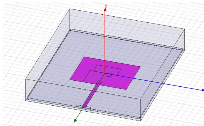
Figure 2 Structure of designed antenna.
