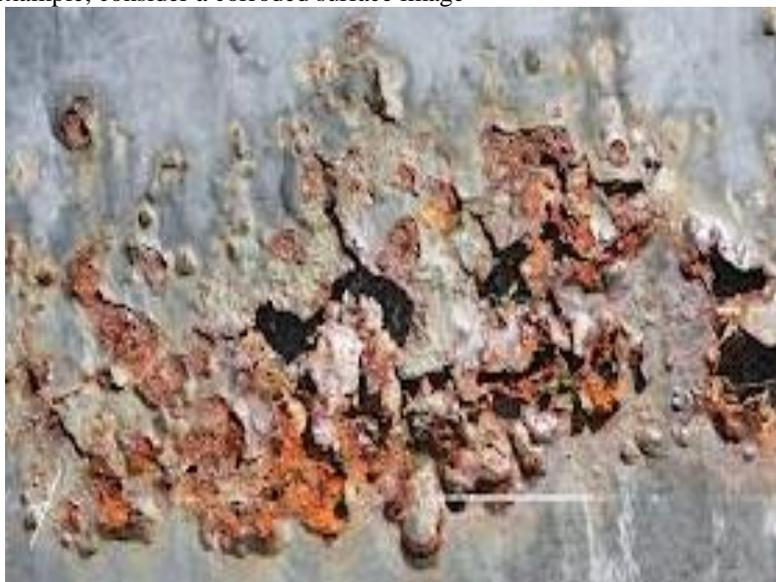
Fig:-Corroded metal sheeting in a marine environment.
