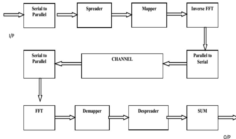
Fig. 1 General MC-CDMA system block diagram
