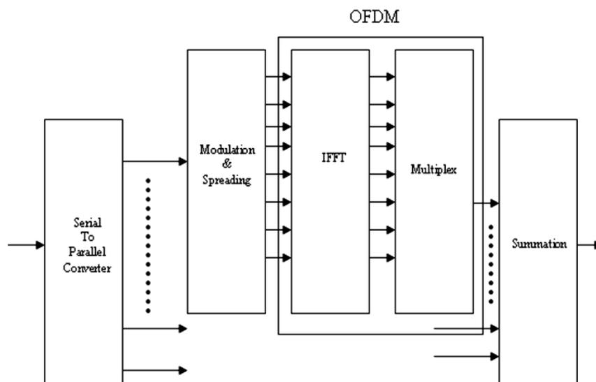
Fig. 2 MC-CDMA Transmitter Implementation
