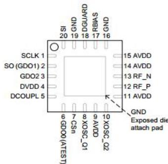
Figure 8. Pin Configuration of CC2500 IR Sensor [10]
