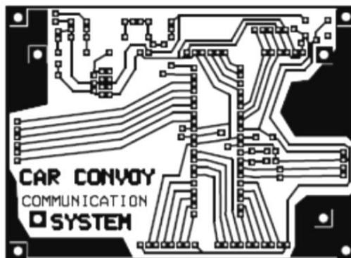
Figure 11. PCB Layout of project module
