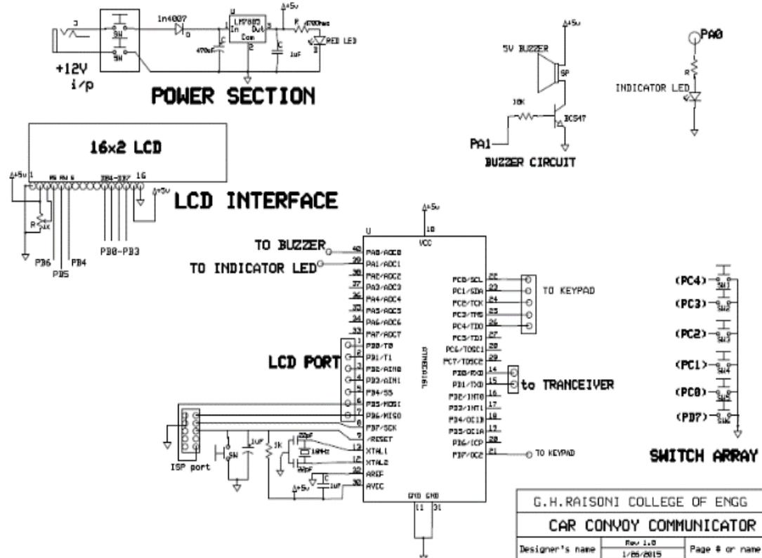
Figure 10. Car Convoy Communicator Circuit Diagram
