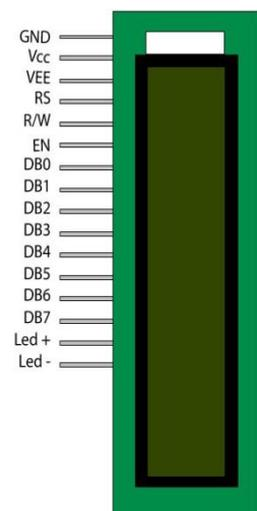
Figure 7. Pin Diagram of 20x4 LCD [18]
