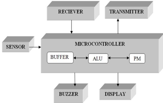
Figure 4. System architecture
