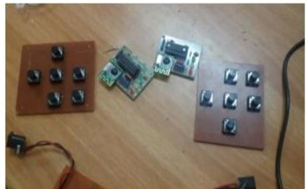
Figure 13. 6 key keypad and Transceiver Module
