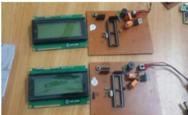
Figure 12. LCD and Microcontroller Module on the PCB
