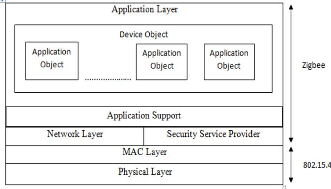
Figure 9. Zigbee Protocol Stack [15]
