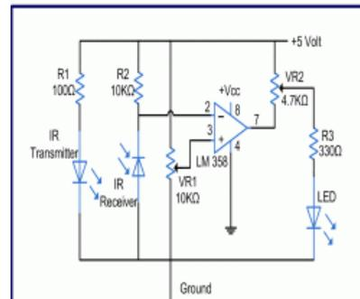
Figure 3.7 Circuit Diagram of an IR circuit [15]
