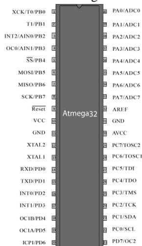
Figure 6. Pin Diagram of AVR ATmega32 Microcontroller [17]
